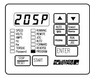
If no faults have occured, Err will be displayed again. If only one fault has occurred, the fault code will be displayed as the first entry in the log. If more than one fault has ocurred, the first entry is the latest fault that occurred.
